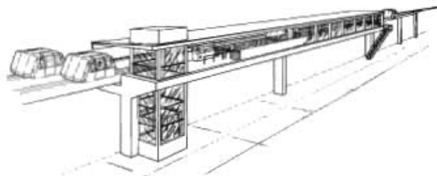
Fig. 3-17. Activity-Center Station Installed Over Curb Line
