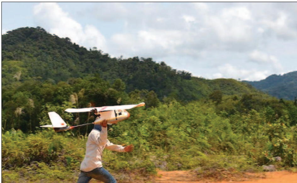
Throwing a drone for “take off.” More cumbersome to use than a multi-copter drone, fixed-wing mini drones are very efficient in vegetation mapping, able to cover a larger area and having safer recovery capabilities from motor power loss. Photo: Yves Laumonier
