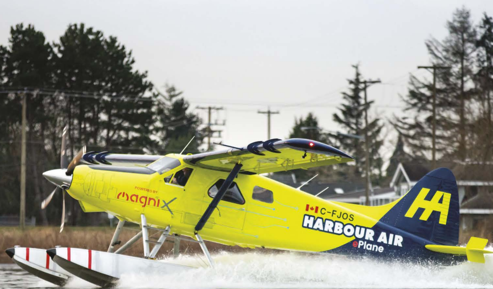
Harbour Air's DHC-2 Beaver takes off with a battery powered electric engine.
