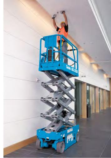
The Genie® GS™-1930 slab scissor lift is easy to maneuver in tight spaces, has a 25-ft working height, boasts quiet electric, zero-emissions operation and is ideal for indoor and outdoor applications on firm, level surfaces.
