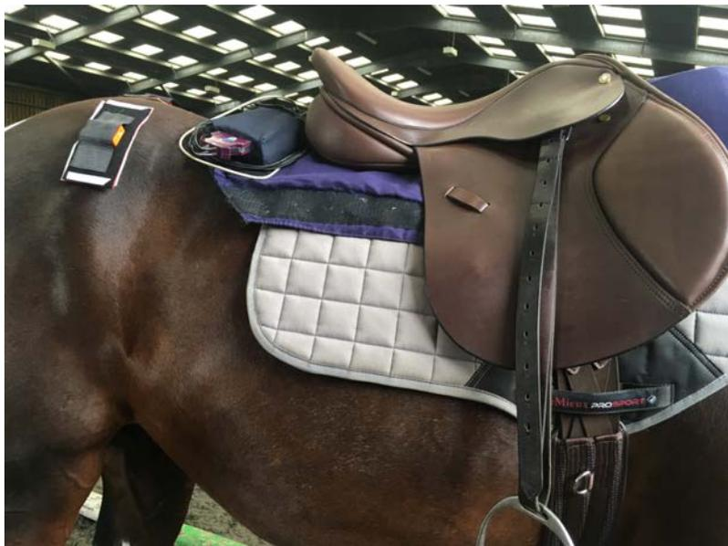
*A calibrated force sensor mat was placed under each saddle*
