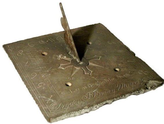
The sundial, one of the earliest scientific instruments, tells time by measuring the passage of the sun through its daily course in the sky. The vast majority of sundials consist of a pointer, called a style or gnomon, and a calibrated plate upon which the pointer casts a shadow.
