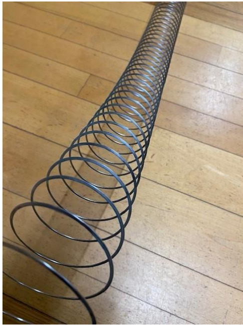
The compressional waves that transfer vibrations and sound become visual with a slinky. This sound slinky is extra long for demonstration purposes.
