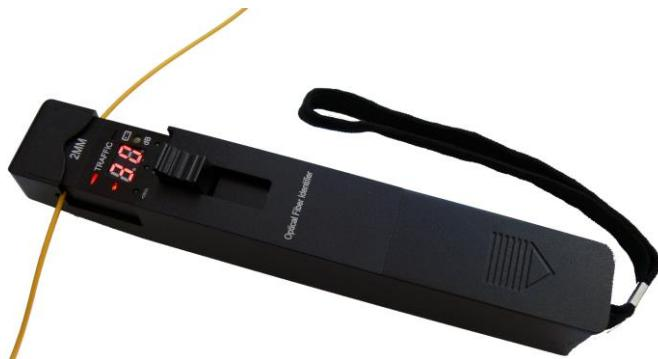
OFI-20A can detect optical signal presence, type and direction anywhere on fibers during a optical network deployment, maintenance or troubleshooting. With non-destructive macro-bend detection technology, it introduces no damage to tested fiber or interference to the service on fiber. OFI-20A is capable of identifying wide-spectrum signals (such as signals in CATV system) and can be used in SONET/SDH & DWDM systems tests.
