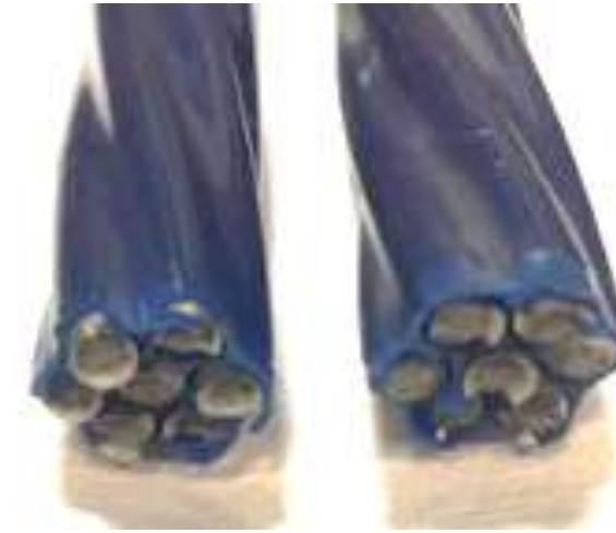
Example tensile test result after 10+ years storage
