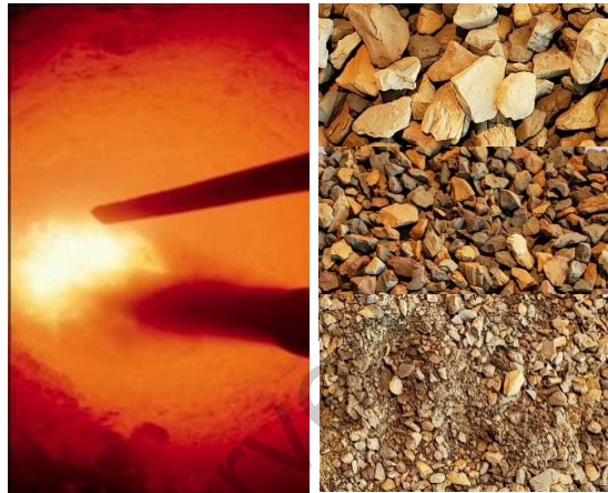
Image courtesy of Norlite (Left: Rotary Kiln Production) FMTEhrani (Right: Expanded Shale, Clay and Slate Aggregates)
