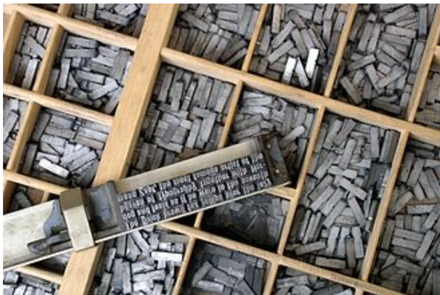
(Moveable type sorted in a letter case and loaded in a composing stick)
