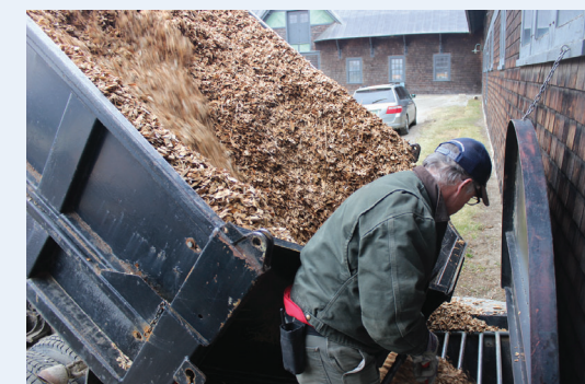
In the winter, a one-ton dump truck delivers wood chips to the boiler system below the Education Center 3-4 times a week.
