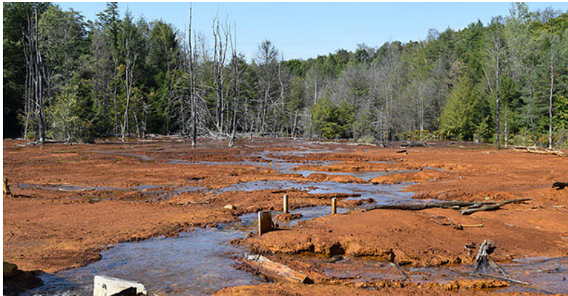
Acid mine drainage welling up from a borehole drilled into an underground mine near Portage, Pa. Dylan Brown/E&E News
