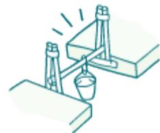
4. Make a load tester by unbending a large paper clip into a V-shape. Poke the ends of the paper clip into opposite sides of a paper cup, near the rim.
