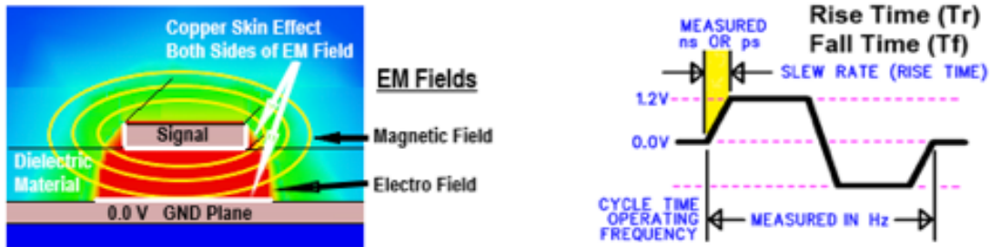
EM Field Between Signal and GND - Square Wave Highlighting Rise Time T_r
