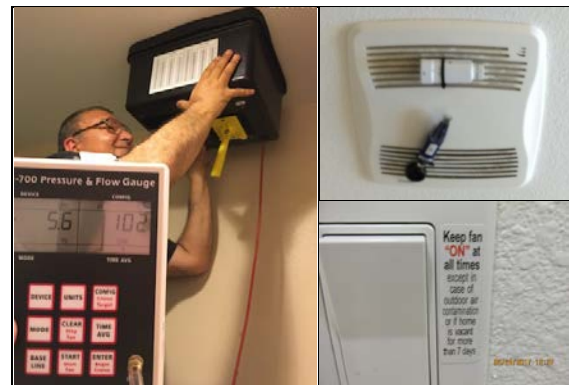
Mechanical ventilation air flow measurement (left), monitoring (upper right), and control label (lower right).
