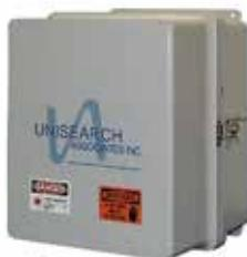
The stack optics are mounted in NEMA-4 enclosures and may be located up to 30m from the analyzer. The temperature range over which the optics can perform to specifications is -40 °C to +60 °C. NEMA 4X and Class I, Div1 or 2 enclosure options are also available.
