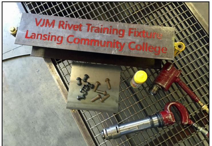
VJM Rivet Training Fixture for rivet training at Lansing Community College
