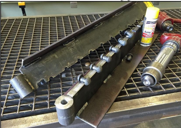
Rivets are ready to remove
