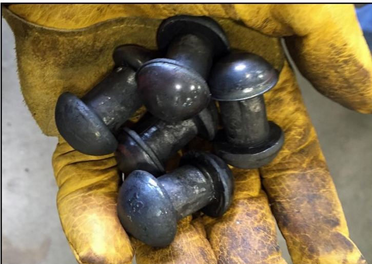
Fully formed rivets can be inspected.
