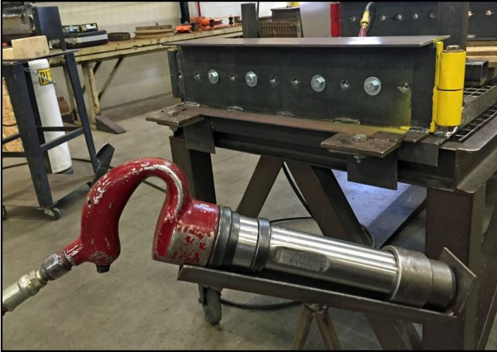
Rivet training fixture bolted in place Fixture is designed for 5/8" round head rivet, 7/8" and 3/4" grip
