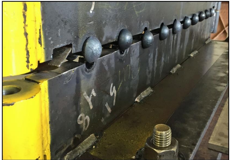
Pry bar is used to separate the two sections of the rivet training fixture
