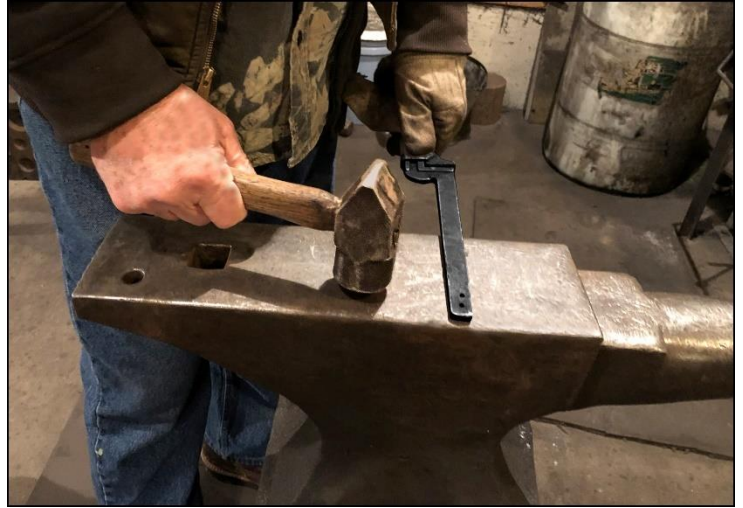
Bernard demonstrates a hammering technique with the short handled heavy hammer popularized by Alfred Habermann, a Czech blacksmith.
