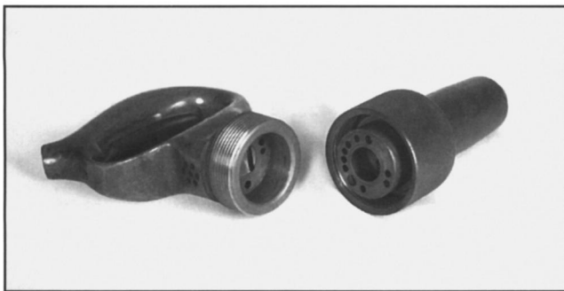
Figure 12. “Little Giant” hammers like these were produced in Chicago by the Standard Pneumatic Tool Company. This bronze example (figure 11), which can still be easily screwed apart to view the valve and piston, bears patent dates ranging from 1883 (Boyer’s original patent) to 1900. Photo by author.
