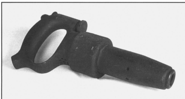
Figure 13. Although the iron hammer is the heaviest of the two, its weight, a little more than 8 lbs., places it in the chipping tool category. The screw on the upper portion of the handle was connected to a bushing that regulated the volume of air entering the hammer. The force of a blow on a hammer without this feature could only be regulated by the degree that the trigger was depressed. This example from the Missouri Historical Society’s collections matches the hammer shown in an 1899 announcement by Standard. Photo by author.
