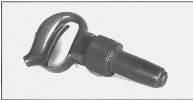
Figure 11. A pair of pneumatic hammers was donated to the Missouri Historical Society in 1929 by a local patent attorney as examples of “very early pneumatic hammers.” They are believed to be the oldest extant in the country. Photo by author.
