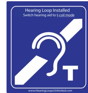
To use the full benefit of the hearing loop please activate your hearing aid by a pressing the T-coil program button on your hearing aid. If your hearing aids have a setting for microphones with T-coil (M&T), the T-coil only setting is recommended.
