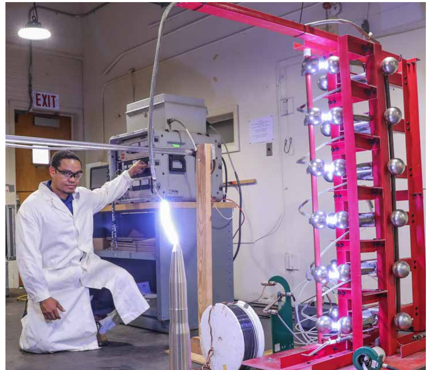
TOP: Naval Surface Warfare Center Indian Head Division ElectroStatic Discharge (ESD) Tech Agent Team Lead observes the transient arc of 300kV to the discharge point between the Helicopter-ESD (HESD) Marx and the INERT ordnance on the ground plane during Bare Ordnance HESD testing. (Official U.S. Navy photo)
