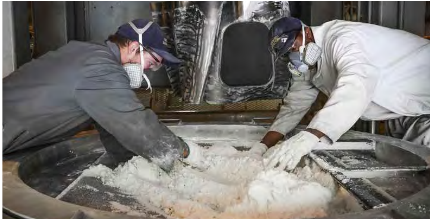
Naval Surface Warfare Center Indian Head Division operators screen energetic material at the 420 Gallon Mixer. (Official U.S. Navy photo)
