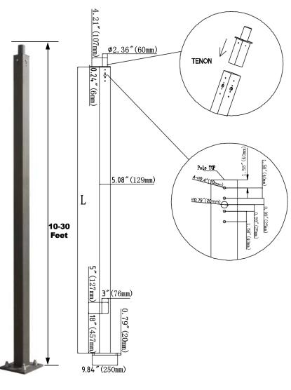
The LPT Series Square aluminum poles are built from high strength aluminum Square tube and are available side drilled for arm mounted area lighting luminaires or with tenon mounts for flood and post top luminaires. Typical area lighting applications include retail centers, industrial parks, schools and universities, public transit and airports, office buildings and medical facilities. Mounting heights of 10 to 30 feet can be used based on selected luminaire application.
