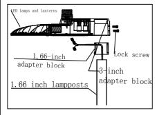
Method 2: install the 3 inch adapter piece on the lamp. then install the 1.6-inch adapter piece on the lamp post, install on the 1.66-inch lamp lever, tighten the two screws, the lamppost is fixed. Lamps of lamps and lanterns can adjust the Angle of lamps and lanterns. (5  $^{\circ}$  / 2.5  $^{\circ}$  $0 \degree / 2.5 \degree / - 5 \degree$ ). (see charts.)
