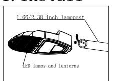
Method 1: the lamps and lanterns directly install the lamp rod, the outer diameter of the lamp pole is 3 inches and 2.4 inches two kinds of specifications. When the street lamp is assembled into the lamp post, the Angle of the lamp will be adjusted according to the actual situation. (5  $^{\circ}\,$  for lamps and lanterns with Angle / 2.5  $^{\circ}$  0  $^{\circ}$  / 2.5  $^{\circ}$  / - 5  $^{\circ}$  ) (as shown)
