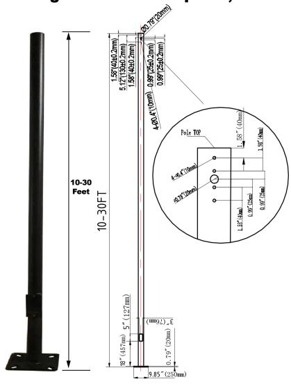
The WISDOM Series Round Steel poles are built from high strength Steel Round tube and are available side drilled for arm mounted area lighting luminaires or with tenon mounts for flood and post top luminaires. Typical area lighting applications include retail centers, industrial parks, schools and universities, public transit and airports, office buildings and medical facilities. Mounting heights of 10 to 30 feet can be used based on selected luminaire application.
