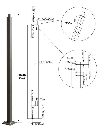
The LPT Series Straight Square Steel poles are built from high strength steel tube and are available side drilled for arm mounted area lighting luminaires or with tenon mounts for flood and post top luminaires. Typical area lighting applications include retail centers, industrial parks, schools and universities, public transit and airports, office buildings and medical facilities. Mounting heights of 10 to 30 feet can be used based on selected luminaire application.
