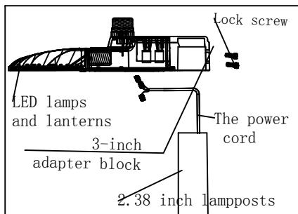
Method 3: when the lamppost is turned into a lamppost 2.38 inches, the lamp is mounted directly on the lamp, with two screws and the lamppost fixed. The Angle of lamps and lanterns adjusts according to actual situation. Lamps and lanterns (5° / 2.5° Angle 0° / 2.5° / -5°) (as shown)
