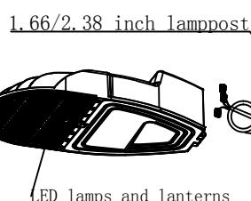
Method 1: the lamps and lanterns directly install the lamp rod, the outer diameter of the lamp pole is 3 inches and 2.4 inches two kinds of specifications. When the street lamp is assembled into the lamp post, the Angle of the lamp will be adjusted according to the actual situation. (5° for lamps and lanterns with Angle / 2.5° 0° / 2.5° / -5°) (as shown)
