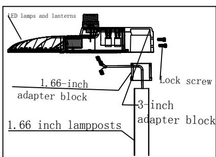
Method 2: install the 3 inch adapter piece on the lamp, then install the 1.6-inch adapter piece on the lamp post, install on the 1.66-inch lamp lever, tighten the two screws, the lamppost is fixed. Lamps of lamps and lanterns can adjust the Angle of lamps and lanterns. (5° / 2.5° 0° / 2.5° / -5°). (see charts.)
