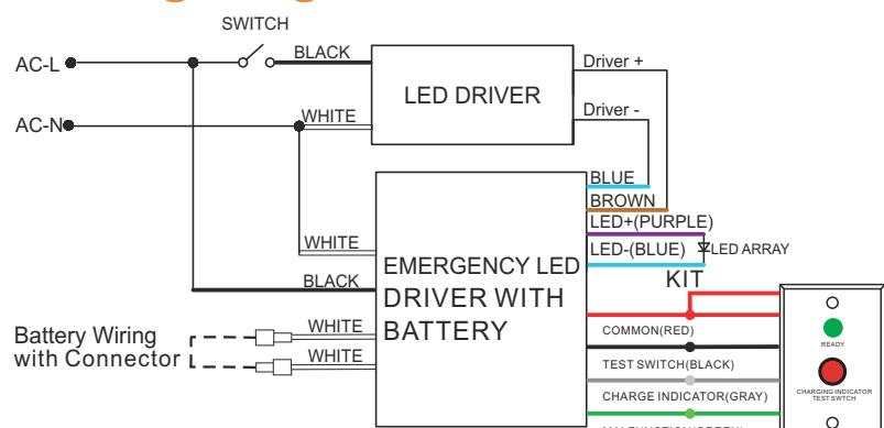
1. DO NOT MATE CONNECTOR UNTIL INSTALLATION IS COMPLETE AND AC POWER IS SUPPLIED.
