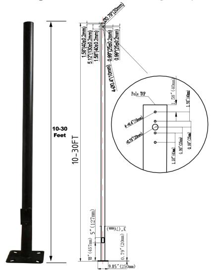
The LPT Series Round aluminum poles are built from high strength aluminum Round tube and are available side drilled for arm mounted area lighting luminaires or with tenon mounts for flood and post top luminaires. Typical area lighting applications include retail centers, industrial parks, schools and universities, public transit and airports, office buildings and medical facilities. Mounting heights of 10 to 30 feet can be used based on selected luminaire application.
