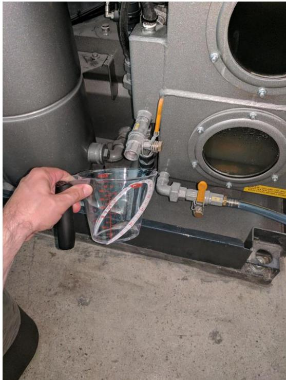
By draining 16 ounces from the bottom of the middle (primary) separator, we remove most of the free water from the bottom of the tank. Use a clear measuring cup like the one shown.
