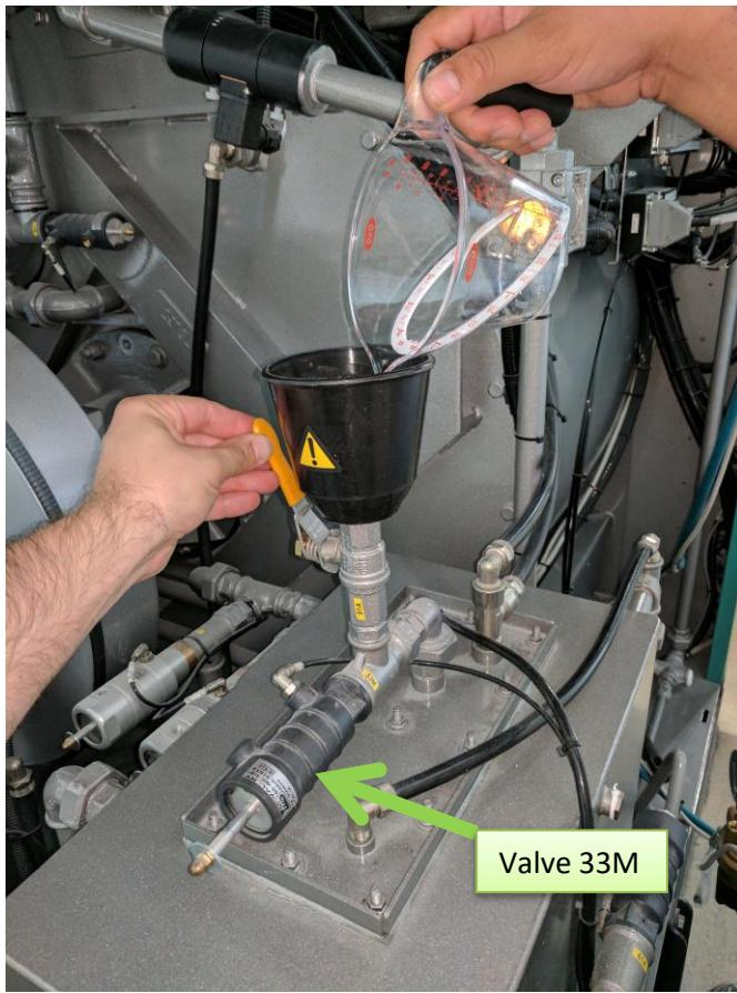
Turn on the machine and push the DOOR OPEN button. This unlocks all the doors as well as opens valve 33M. Hold open the yellow ball valve and pour the 16 ounces back into the separator. It will go into the Primary Separator.
