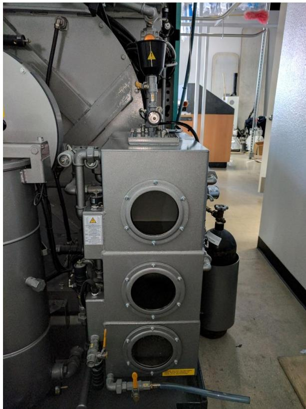
This separator included a new feature where the machine can drain the Primary and Secondary separators into the still, and then rinse out the separators using a jet spray built inside the separator tanks.
