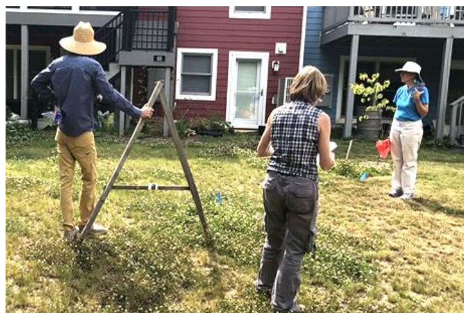
Determining where to dig. Michael Judd from Ecologia Design is holding an A-frame, used to locate the contours of the land. Each contour line point will be marked with a flag. SV members Charlotte and Kay are learning how this works.
