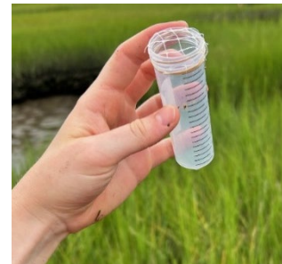
Sediment traps, made with small centrifuge tubes and netting to keep out snails and crabs, are inserted in the marsh surface.
