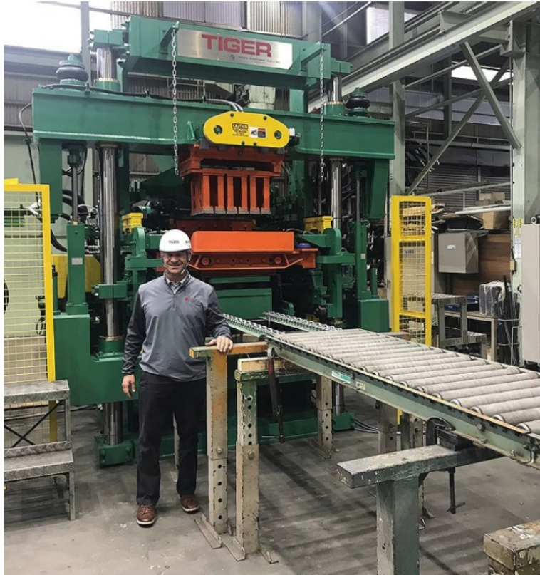
Tiger founder Yutaka Kitahara (top, right) applied farm machinery production competencies to concrete block equipment in 1963. Evolution of block and paving stone models, plus companion unit handling and finishing equipment, have positioned the manufacturer among global concrete masonry machinery brands. Current offerings include the Tiger Model S-3, seen here, with Sam Lock, Regional Operations Manager, Midwest Block during a visit of the Tiger facility in Japan.
