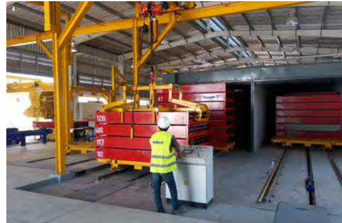
1 The reinforcement wires are semi-automatically prestressed with a tensioning force of 460 kN 2 Electrically driven discharge screws pour the concrete into the mould with high precision 3 Turning crosshead for the demoulding process 4 A lifting traverse in the exit area of the curing chamber
