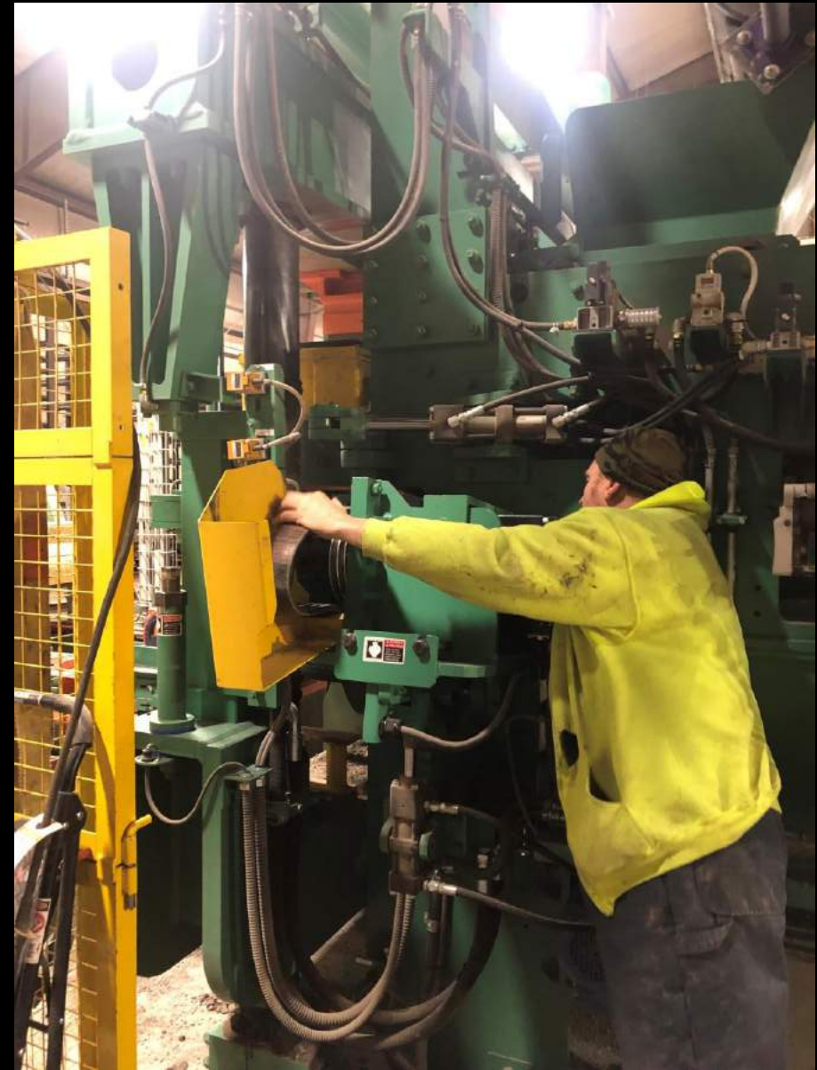
Re-Installing Vibrator Belts
