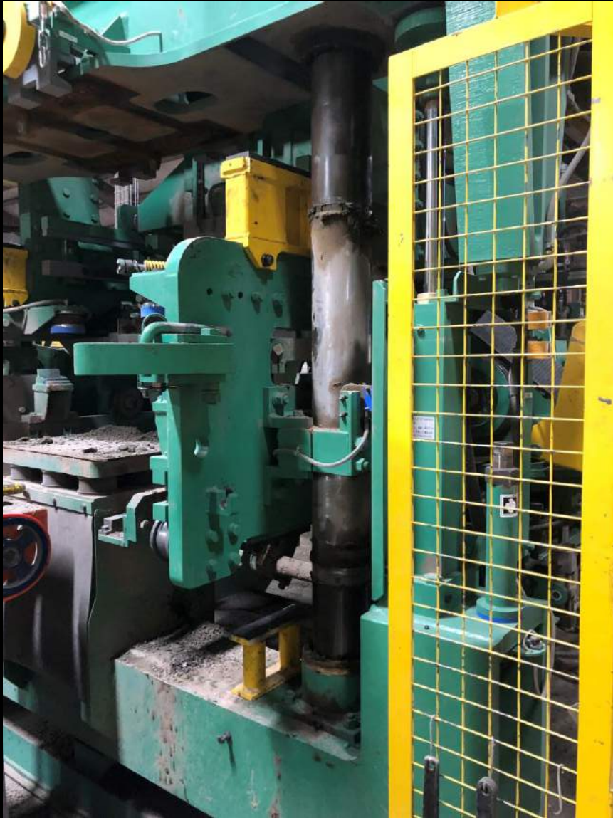
Upper & Lower Height Stops Replaced For 6" High Units
