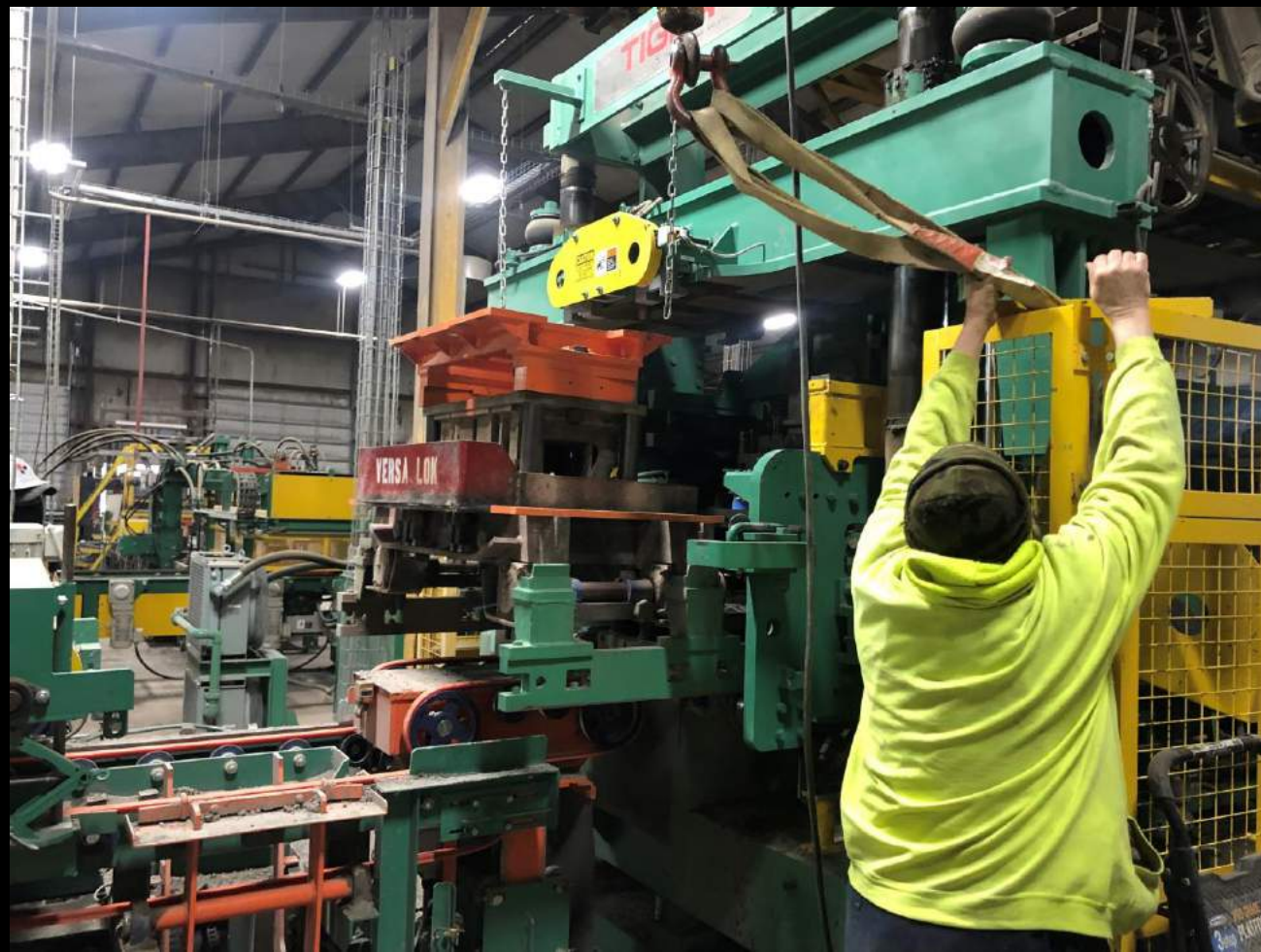
New Mold In Cradle And Being Installed
