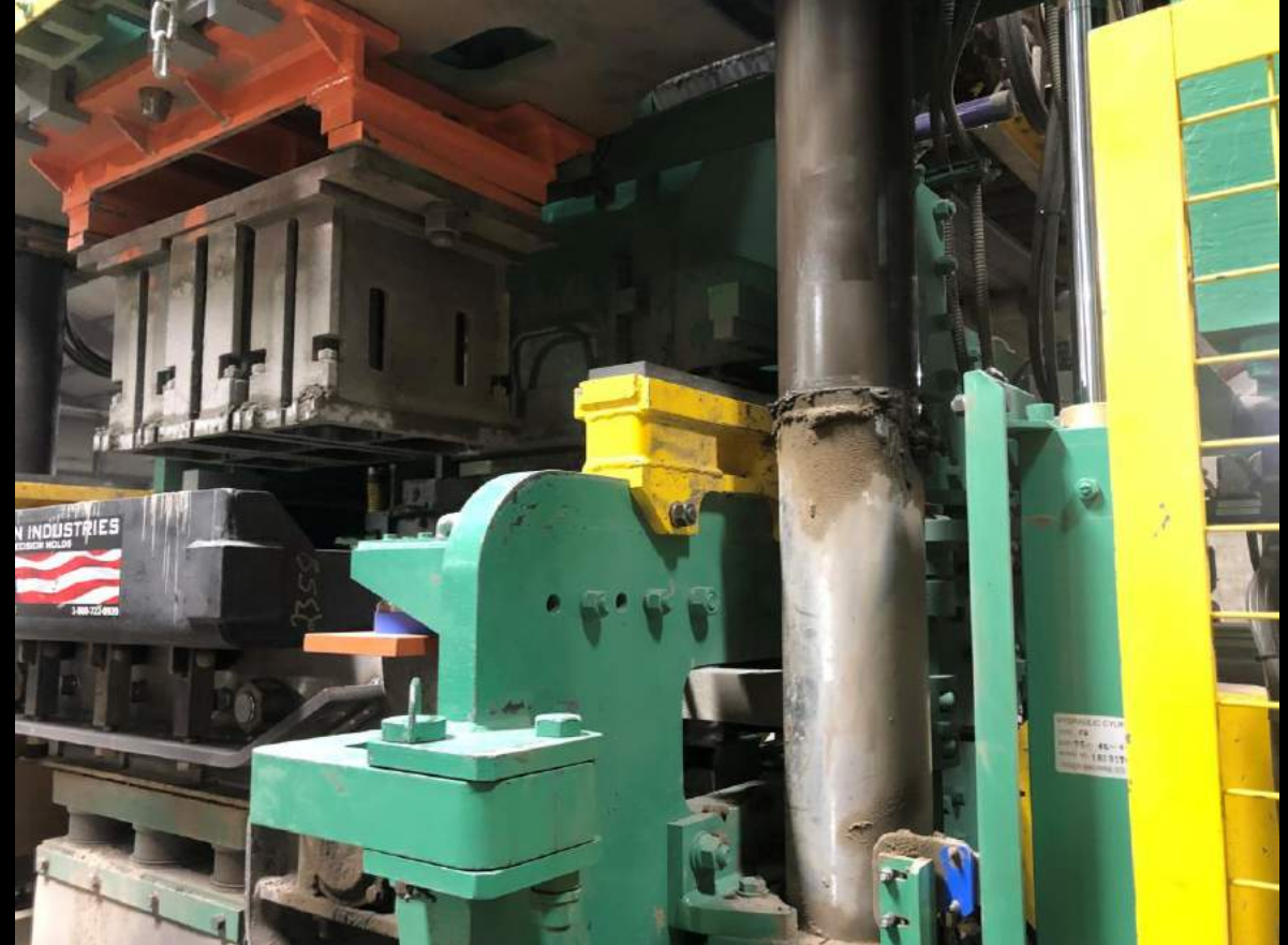
Upper Height Stop For 7-5/8" High Units
