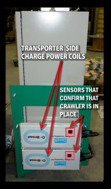
The crawler and transfer car use positional sensors to ensure that the crawler is in the proper location to allow for wireless charging.
