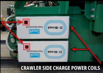
Inside of the crawler, the electrical cabinet is the charging device and display for errors and charging status.
