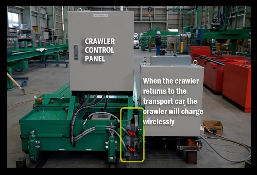
When crawler is back at transporter, (reverse end of crawler) the charger device will be activated and the coil will operate to charge the crawler battery.
