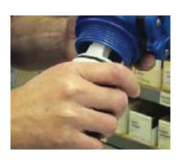
Step 5: You can also test by taking the stem, inserting the plunger, and pulling it out. It should make a pop sound. If it doesn't make a pop sound or if you see damage, it is time to replace the plunger seal.
