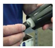
Step 15: Next, take the check valve nut and thread it back onto the stem.It may be a bit snug, but it will slide out.
