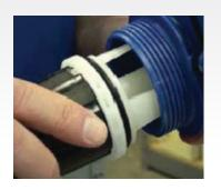
Step 16: Insert the plunger into the housing, press it in as far as it will go, and twist ¼ turn clockwise to lock.
