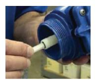
**Step 19:** Hand-tighten the stem nut.
