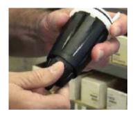
Step 7: Pull the check valve straight out.
