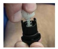
Step 9: Once you have the parts out, ensure they are not damaged, gummy, sticky, or missing. If the parts are dirty, you can reinstall them. If they are damaged or missing, it's time to replace them. Remember to keep these parts clean and in good shape to ensure your check valve will do its job.
