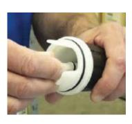
Step 3: Next, grasp the plunger and twist it ¼ turns counterclockwise. Pull straight out to remove.
