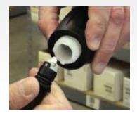
Step 11: Slide the spring over the top of the neck of the cone.
