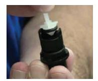
Step 14: Reinstall the check valve into the stem.
