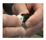
Step 12: Replace the retainer by aligning it and turning it a ¼ turn clockwise to lock.
