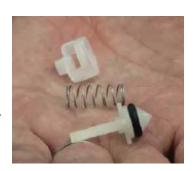
Step 13: Pull on the top before reinstalling the check valve to ensure it stays together.
