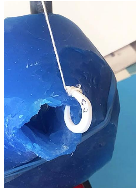
Figure 3. 3D-printed hook replica “catching” the silicone fish mouth model.
