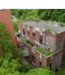
**#9 Rochester Garbage Disposal** - Below the bridge, on the west side of the gorge, is an abandoned garbage incinerator with a tall smokestack. This area of the Genesee River gorge was used to sort, recycle, and burn Rochester's trash, beginning in 1910. The steam produced by the boiler was supplied to nearby buildings and factories.
