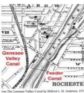
**#12 Feeder Canal** - You're walking on what was once the Lehigh Valley Railroad bed, which was located between the Genesee River and a "Feeder Canal". The Feeder Canal fed water from the Genesee River into the Erie Canal in downtown Rochester. It also provided a detour for canal boats, in case the Broad Street Aqueduct was broken.
