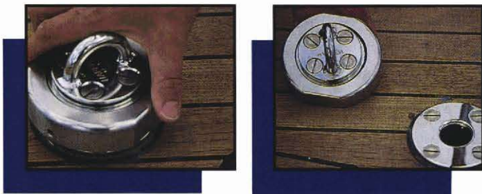
Removable padeye. As padeye is unscrewed, filler plug automatically fills hole to make fitting flush.
