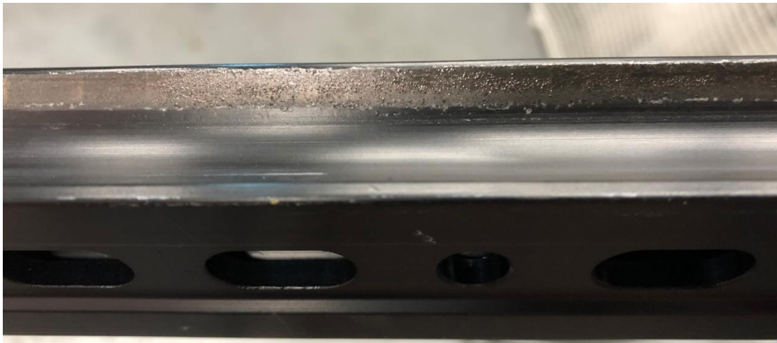
Bronze rollers wore away the anodizing and left containment particles
