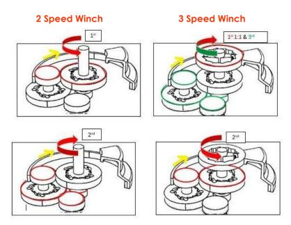
An example of how 2 and 3 speed winches operate is below, the Yellow arrow indicates the drum direction,
