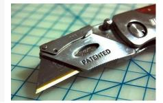
There have been cases where workers have suffered injuries from exposed blade tips. This is because the blades did not completely retract into the handle. That's why it's important for workers to use the proper size blades or replace defective retraction mechanisms. Some companies use self-retracting utility knives – the blade automatically retracts when not in use. The following are safety precautions to keep in mind when using utility knives:
