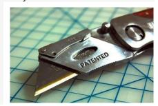
There have been cases where workers have suffered injuries from exposed blade tips. This is because the blades did not completely retract into the handle. That's why it's important for workers to use the proper size blades or replace defective retraction mechanisms. Some companies use self-retracting utility knives – the blade automatically retracts when not in use. The following are safety precautions to keep in mind when using utility knives:
