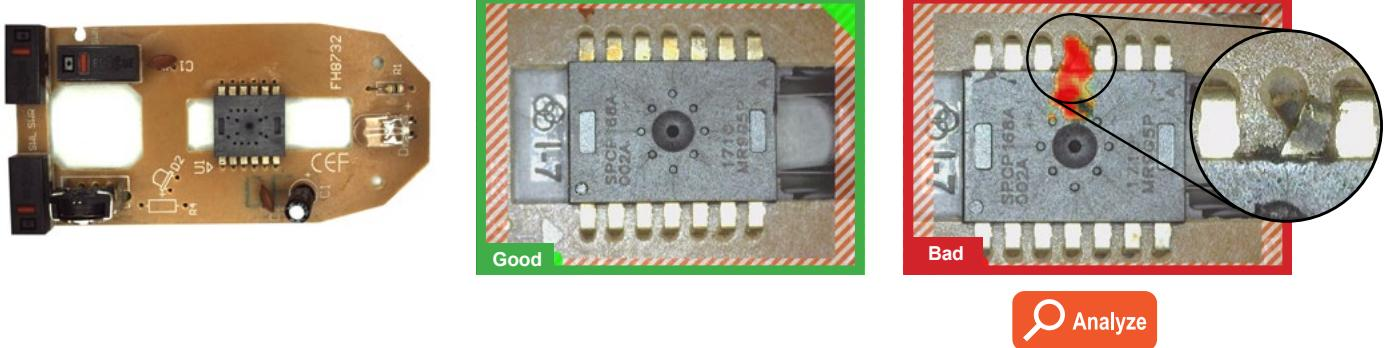
*ViDi Red-Analyze identifies defective pins on an IC.*
