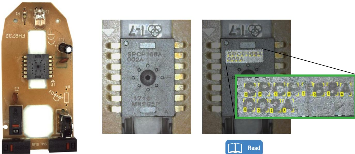
*ViDi Blue-Read recognizes deformed characters on a chip despite image formation issues.*
