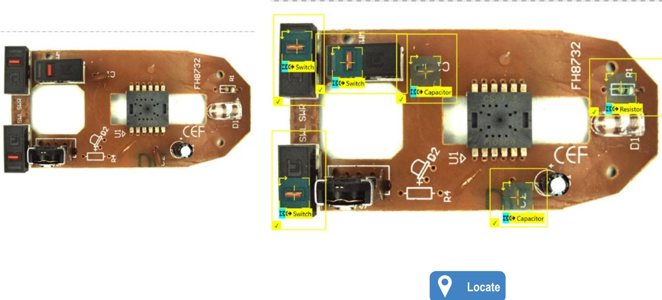
*ViDi Blue-Locate identifies and counts components on a PCB.*
