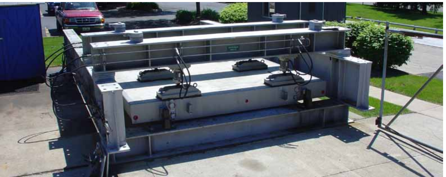
The weighbridge module lifecycle testing machine used by METTLER TOLEDO replicates the forces of trucks driving over the scale.
