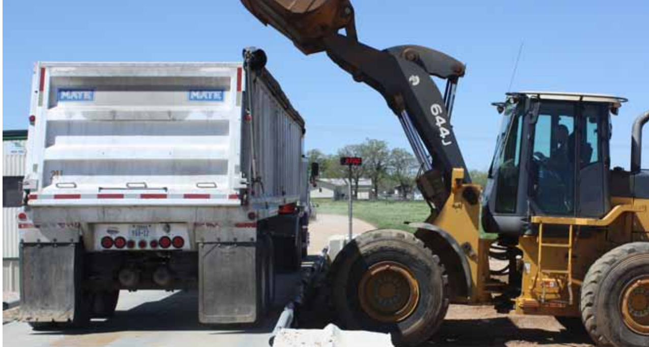
With a remote weight display mounted in view of the loader operator, this truck can be filled to the maximum road-going weight limit
