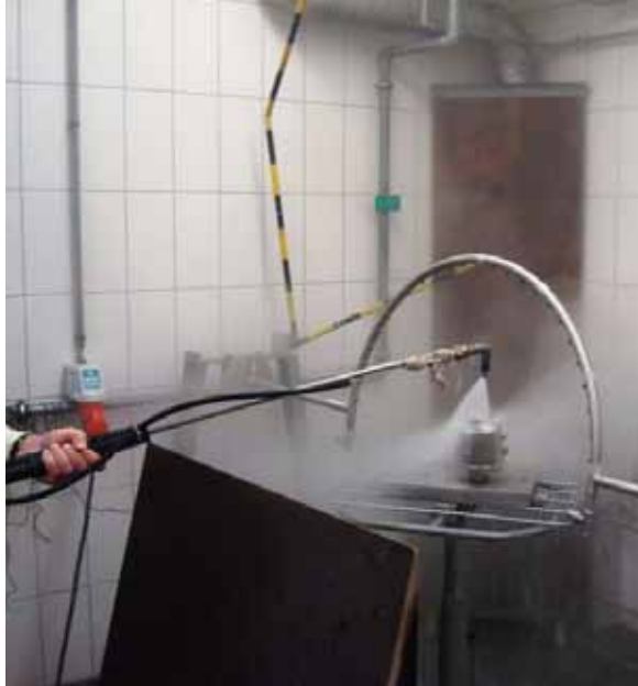
A POWERCELL® PDX® load cell undergoing an IP69K test with pressurized spray
