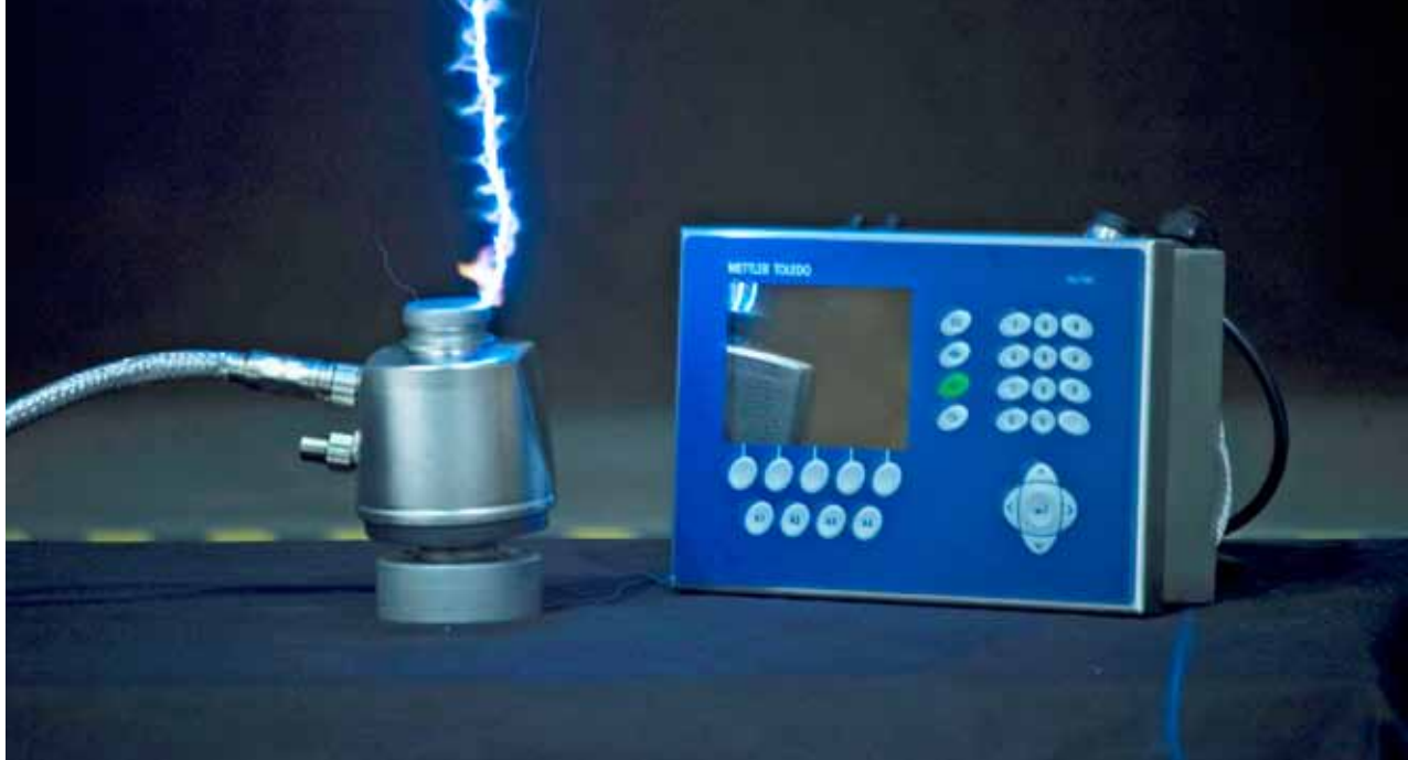
A POWERCELL® PDX® load cell connected to an IND780 terminal during a lightning test
