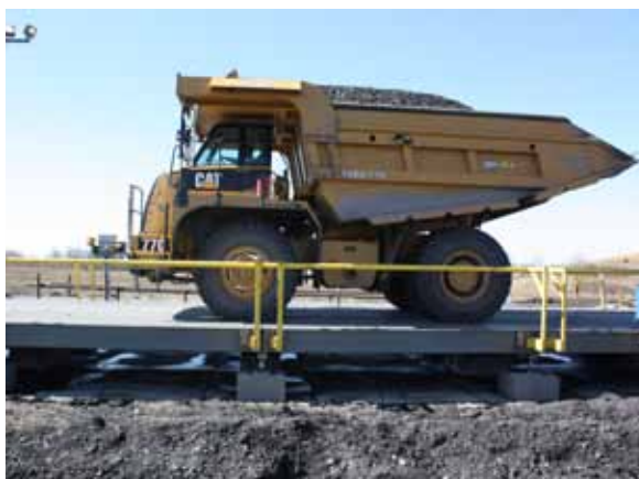
An open-sided scale design can aid in serviceability
