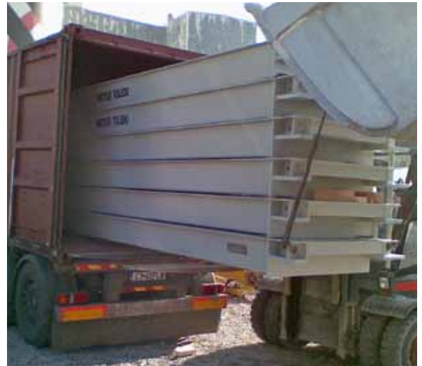
Some manufacturers can offer containerized scales to simplify transporting the scale long distances, or to remote areas
