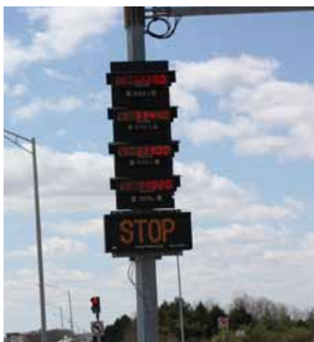
A roadway weigh station uses multiple remote displays to show drivers the weight of each dual tandem axle, as well as the total gross weight of the truck
