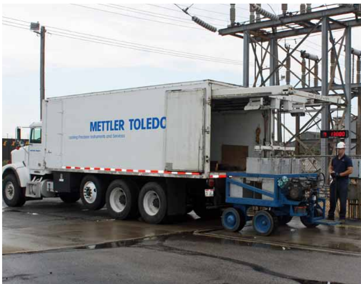
A calibration check can be performed with large test weights that are loaded onto a motorized cart. The technician moves the cart to various points on the scale with different amounts of weight to test for consistent accuracy from the scale
