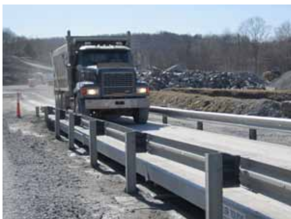
Aggregates sites, for example, may find an open-sided scale easy to clean from spilled product
