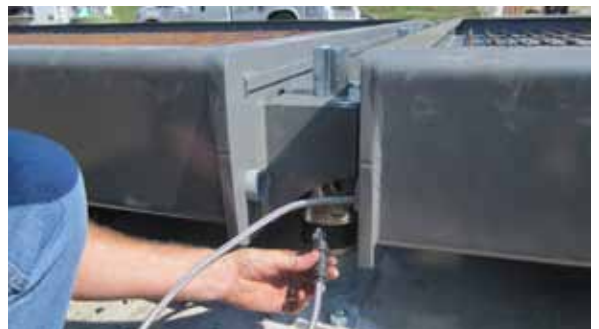
Load cell cables are routed through the scale and attached to the load cells
