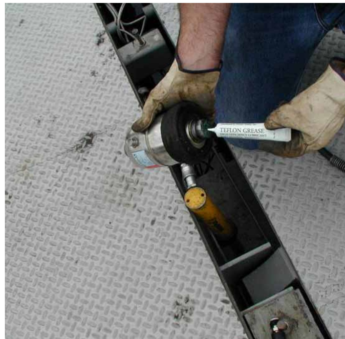
Some areas, such as load cell mating surfaces, require periodic lubrication
