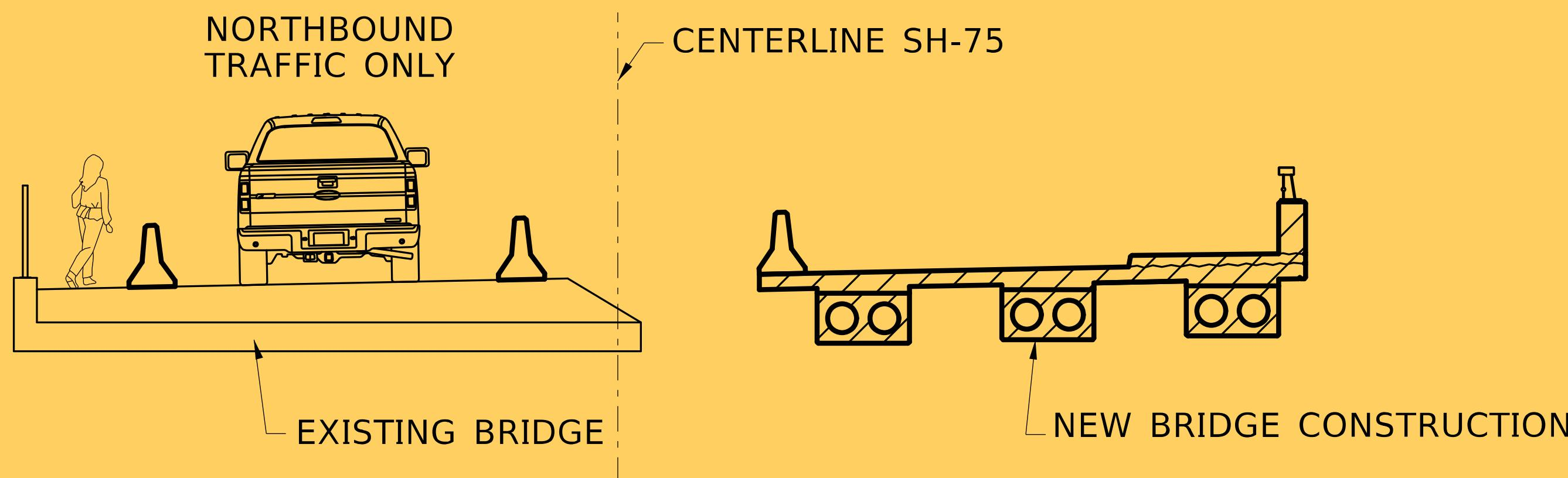
**Between Phase 1 and Phase 2** Between the two construction phases, northbound traffic will drive on the newly constructed part of the bridge while southbound traffic will drive on the existing part of the bridge.
