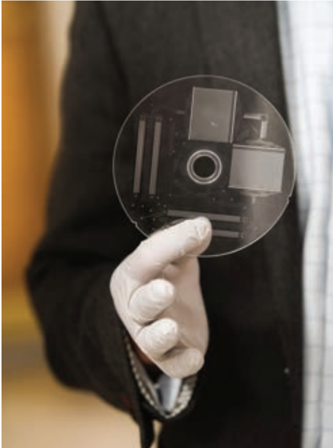
The CTC chip looks like a DVD movie disc but with two tubes attached and a series of tiny channels embedded in it. Photo by Joshua Touster
