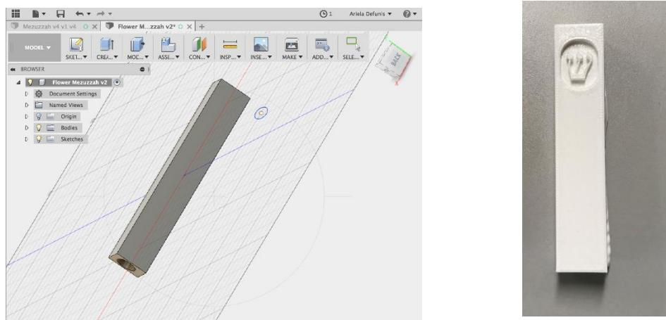
After printing their first model, students assessed some of the challenges with the model, and discovered it was too short to fit in a Mezuzah scroll, had no way of sticking on to a doorpost, and had an exposed hole on the bottom where the scroll went in, suggesting the scroll could also fall out!
