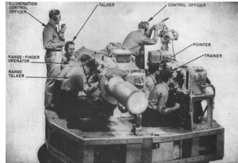
Figure 4: The Mark 37 director. Mounted atop the pilot house on a steel cylinder 9 feet in diameter, the director operated with a staff of seven. (U.S. Navy)
